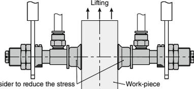
Consider to reduce the stress against holders and pads by sucking the both sides of work-piece.
